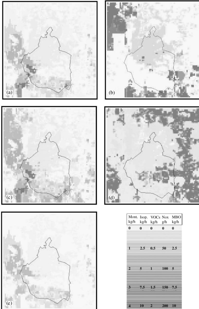
Fig. 5. Spatial distribution of biogenic emissions using  $1 \times 1 \text{ km}^2$  grid cells for monoterpenes (a), isoprene (b), OVOC (c) and MBO (e) emissions in ( $\text{kg h}^{-1}$ ), and for NO (d) emissions in ( $\text{g h}^{-1}$ ), using the climatic conditions of a June day at 14:00h with 10% of cloud cover.
