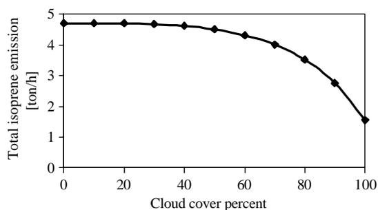
Fig. 7. Isoprene emissions in Mexico Valley as a function of the cloud cover percentage, and considering a constant PAR of  $800 \mu\text{mol m}^{-2} \text{s}^{-1}$  and an environmental temperature of  $20^\circ\text{C}$ .
